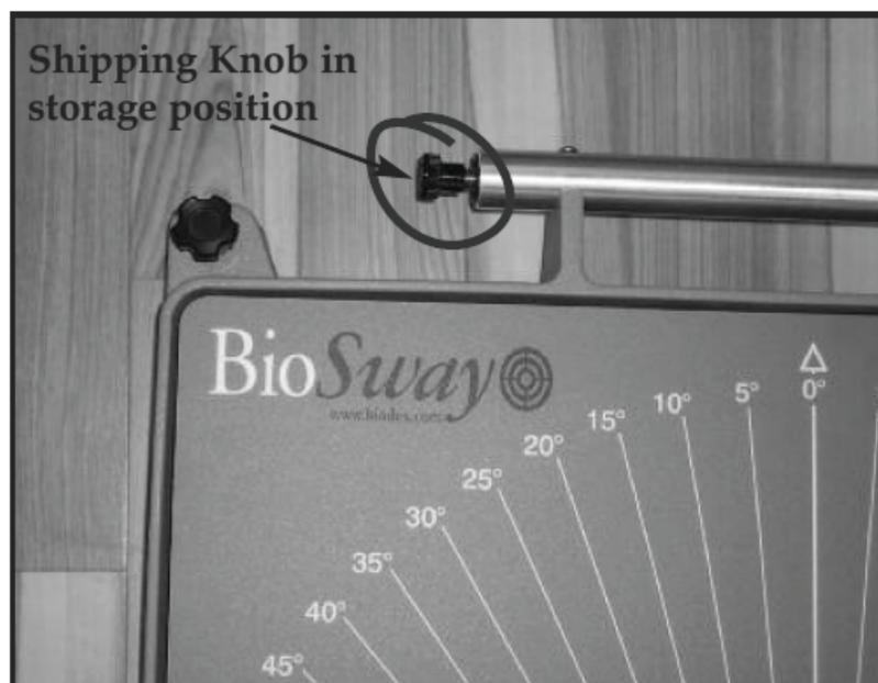
Figure 2.2. Shipping Knob in Storage Position
