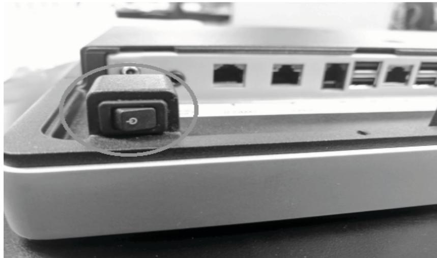
Figure 4.2. Use the rocker button on bottom of the monitor to power the device back on.
