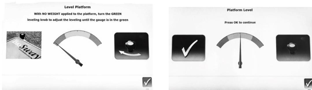
Figure 2.8. When all four boxes on the display are green, the platform is level.
