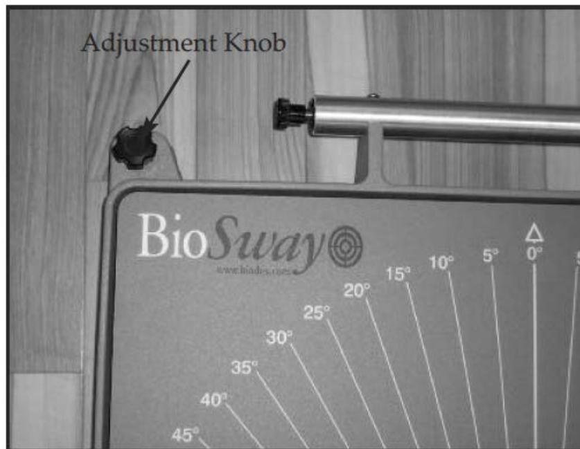
Figure 2.7. Use the Adjustment Knob to compensate for floor irregularities when leveling the platform.
