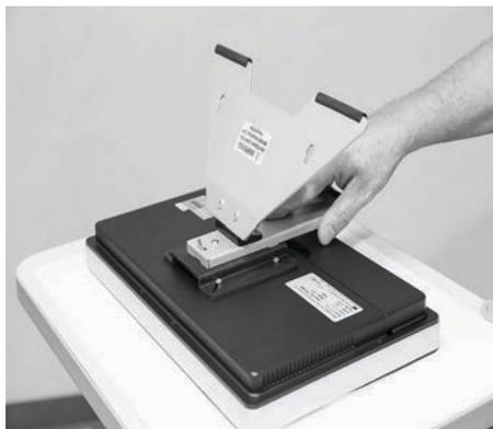
*Figure 2.13. Connecting to the Table Top Stand*
