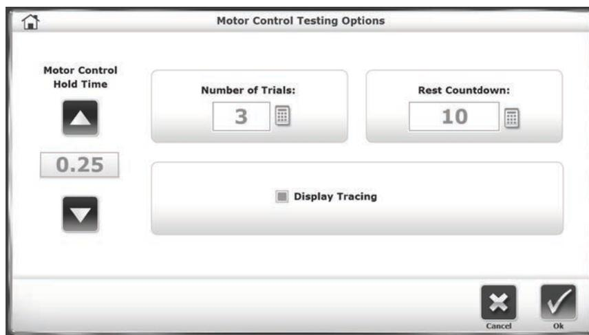
Figure 6.13. The Motor Control Testing Options Screen.
