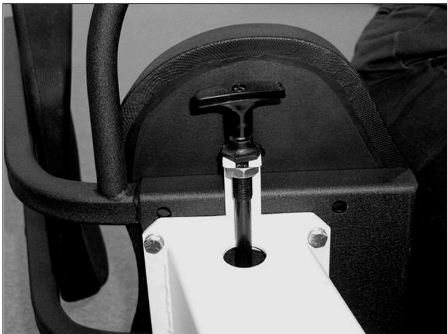
Figure 7. Seat Slide Release Assembly removal.
