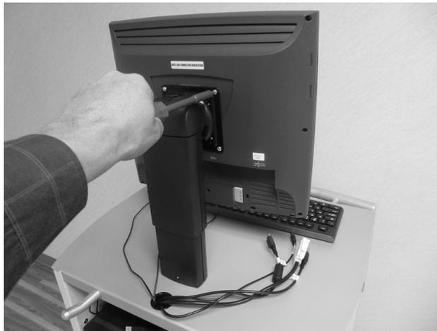
*Figure 4. Removing the Mounting Screws.*
