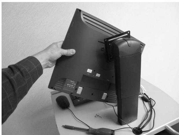
*Figure 5, Removing the Monitor from the Stand.*
