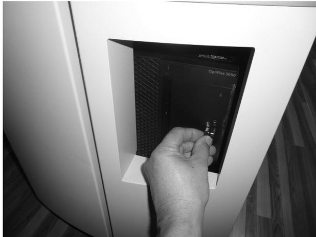
*Figure 39. Installing Wireless Dongle into USB Port on the PC.*
