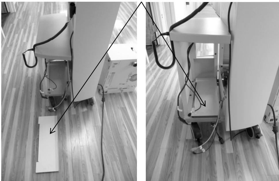
*Figure 18 and Figure 19. PC Adapter Bracket Installation.*
