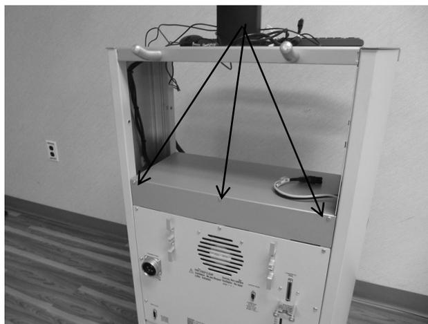
**Figure 10. Cart Illustrating Screws to be Removed.**
