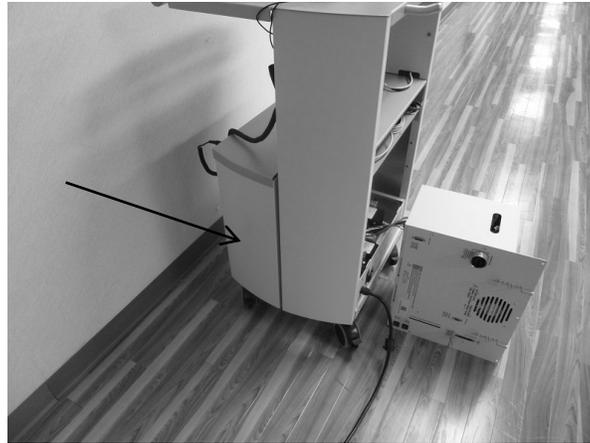
*Figure 14. Side Cover to be Removed.*
