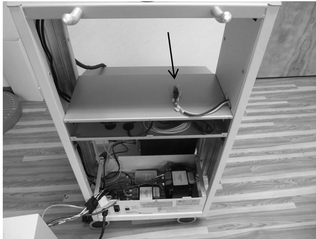
*Figure 32. Cables Routed Inside Power Strip Compartment.*
