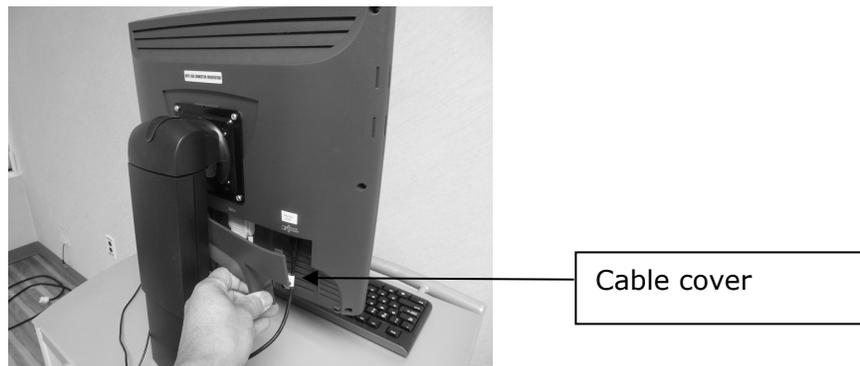
*Figure 2. Removing Cover from Back of Monitor.*
