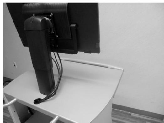
*Figure 26 and Figure 27. USB and HDMI Cables Installed Under the Table Stand Bracket and Tie Cables.*
