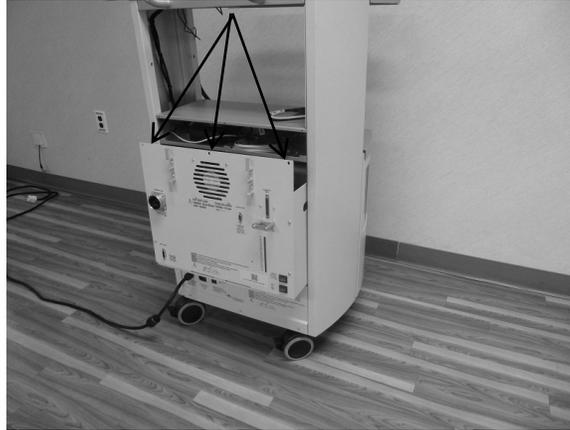
*Figure 12. Controller Drawer Illustrating Screws to be Removed.*
