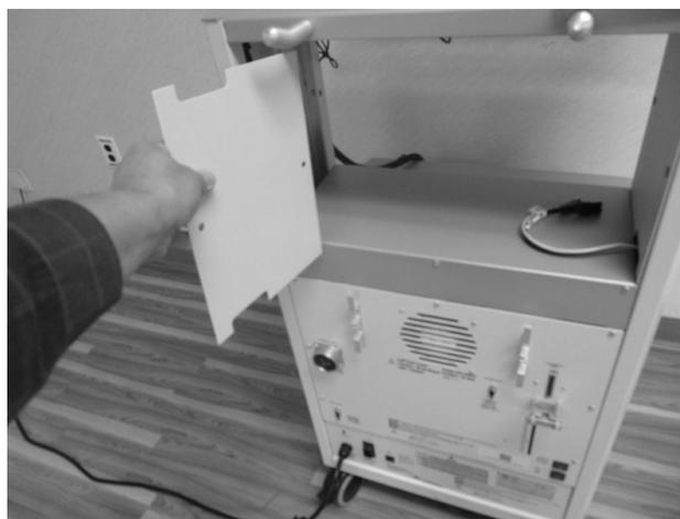
*Figure 8. Removing Cover from Left Side of Cart.*
