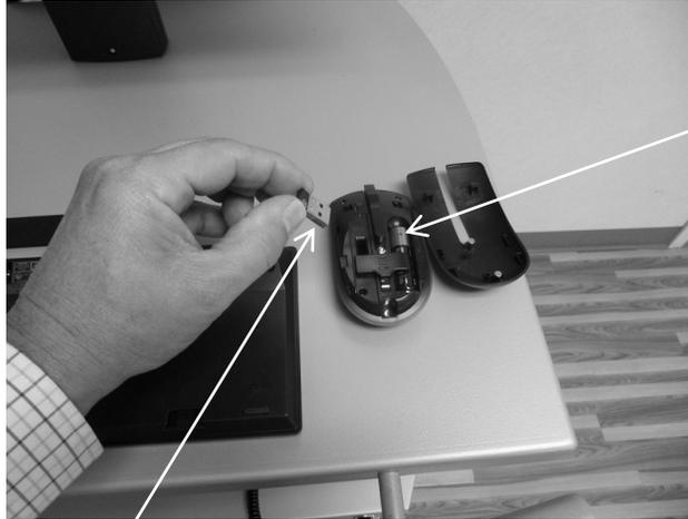
*Figure 38. Battery Installed in Mouse and Wireless Dongle Being Removed.*
