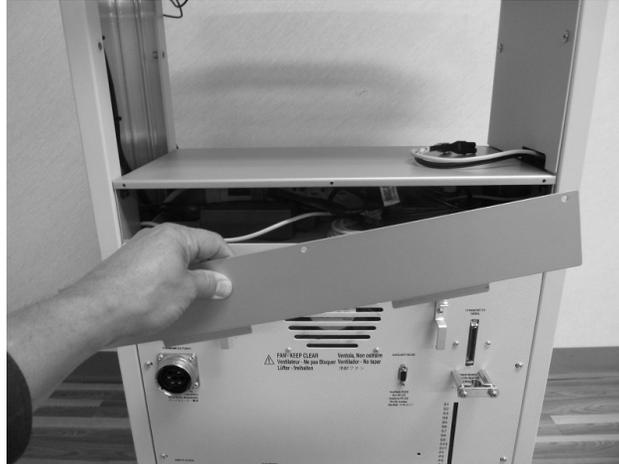
*Figure 34. Power Strip Plate Installation.*
