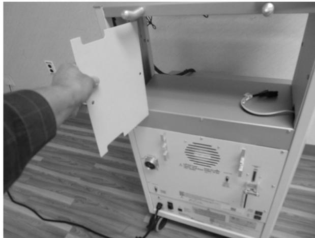
*Figure 35. Side Plate Installation.*
