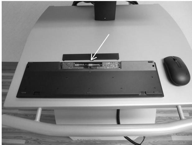
*Figure 37. Battery Installation*
