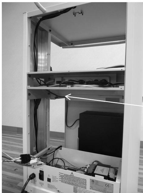
*Figure 31. Final Tie for HDMI Cable.*
