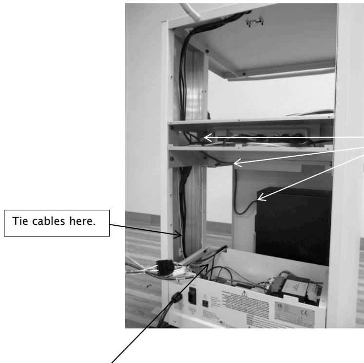
*Figure 30. Cable Routing and Tying.*
