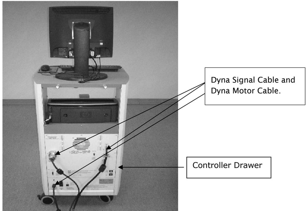
*Figure 1. Rear View of Monitor and CDS Cart.*
