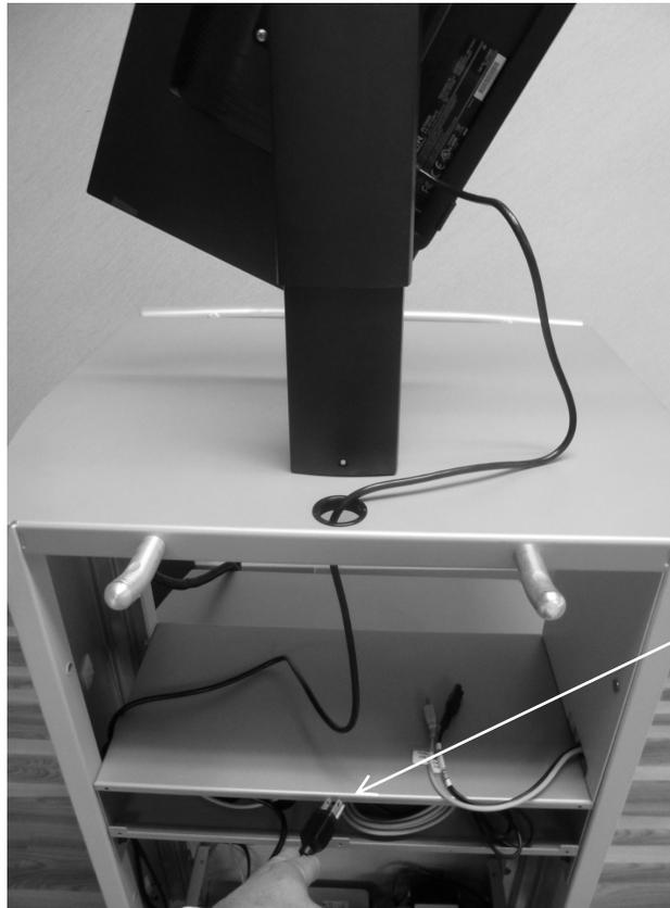
Plug the monitor power cable into the CDS cart power strip.
