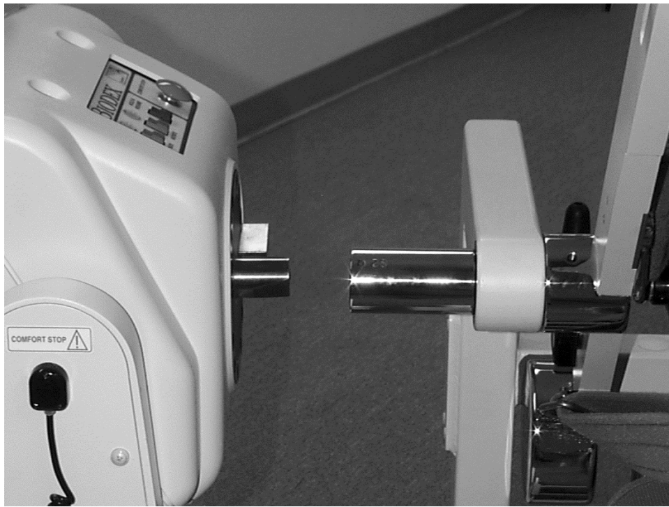
Figure 3.3. Align the Connecting Hub Red Dot with the Dynamometer Shaft Red Dot.
