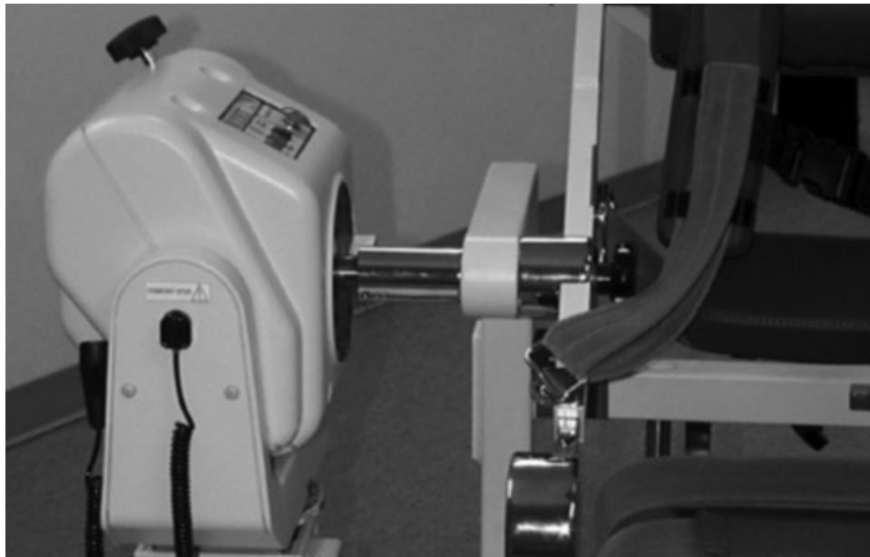
Figure 3.4. Tighten the Connecting Hub Lock Knob to Draw the Back Attachment Securely to the Dynamometer.
