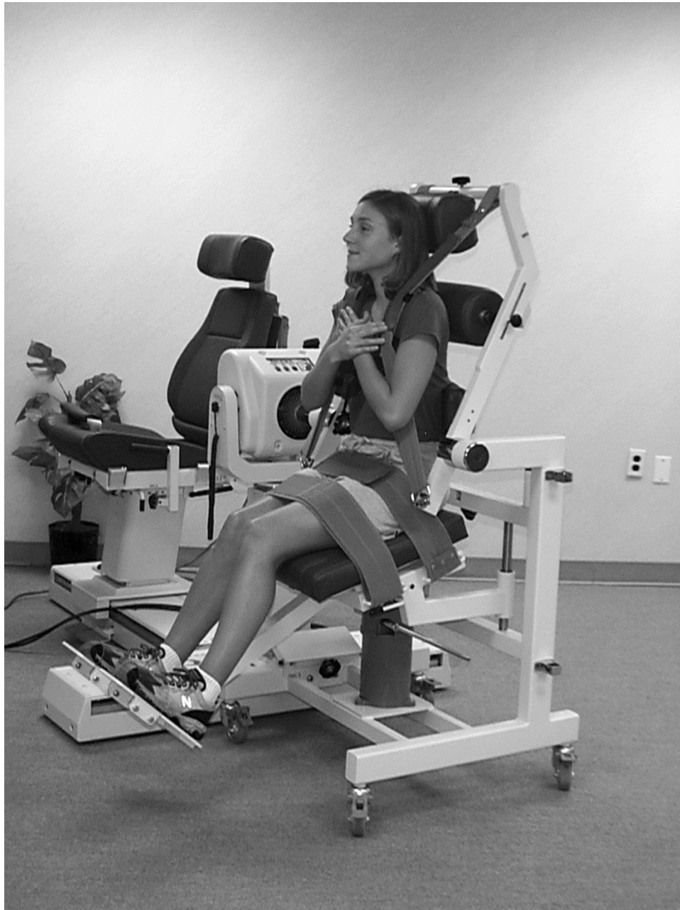
Figure 4.1. The Dual Position Back Ex/Flex Attachment and Multi-Joint System with a Patient in the Semi-Standing (Functional) Position.
