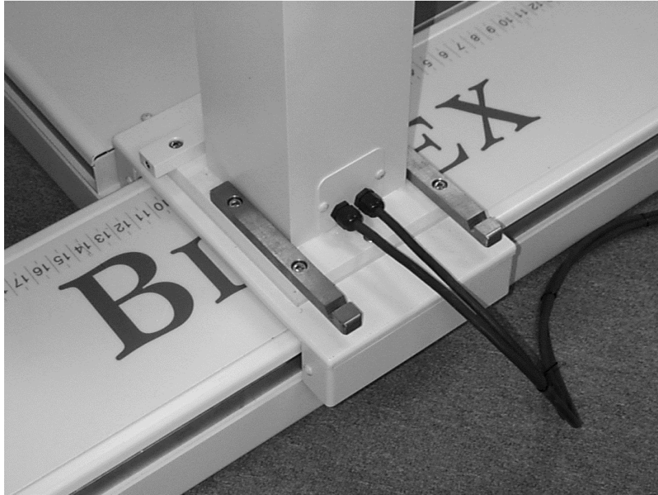
Figure 3.1. The Ex/Flex Mounting Bars Installed on the Dynamometer Base.
