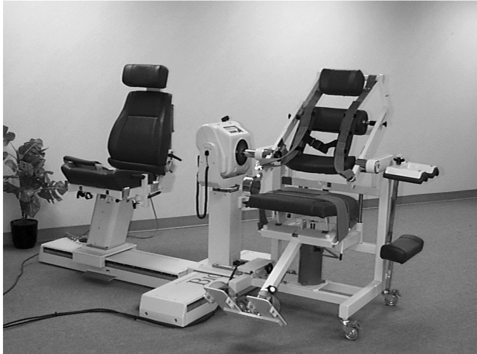
Figure 3.2. The Dual Position Back Ex/Flex Attachment Secured to the Multi-Joint System.
