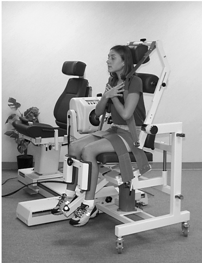
Figure 4.2. The Biodex Dual Position Back Ex/Flex Attachment and Biodex Multi-Joint System with the Patient Seated in the Compressed (Isolated Lumbar) Position.
